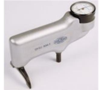
The Barcol Impressor meets the following ASTM (American Society for Testing and Materials) standards: E140-97; D2583-75; B648-78: E140-97 Standard Hardness Conversion Tables for Metals; D2583-75 Standard Method of Testing for Indentation Hardness of Plastics by means of a Barcol Impressor; B648-78 Standard Method of Testing for Indentation Hardness of Aluminum Alloys by means of a Barcol Impressor.
